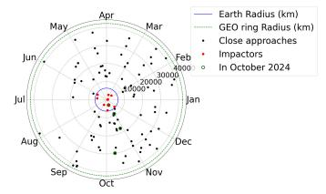
Polar plot representing the geocentric distance of known close approachers versus the time of the year when the close approach happened, extending from the Earth to the Geostationary ring.
