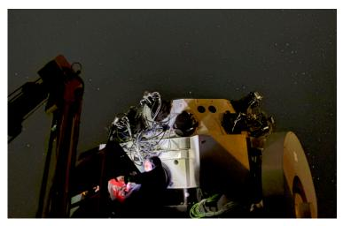
ESA's upcoming wide-field survey telescope, the Flyeye-1, is currently undergoing on-sky commissioning in Matera this summer. The photo shows engineers on the crane performing the camera alignment.
