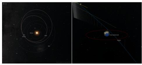
In image to the left, the orbit is reported – showing how it will be affected by the close flyby. In image to the right, the flyby trajectory (blue line) and a geostationary orbit (red line) are visualised. N.B.: the size of the object has been magnified.
