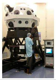
First optical tests of the fly-eye telescope breadboard have started at Compagnia Generale per lo Spazio S.p.A., funded by Italy. The image on the left shows the optical tube, with a 1-meter effective aperture mirror at the bottom, the secondary cage on the top. For the test, the instrument is equipped with two identical optical channels.
